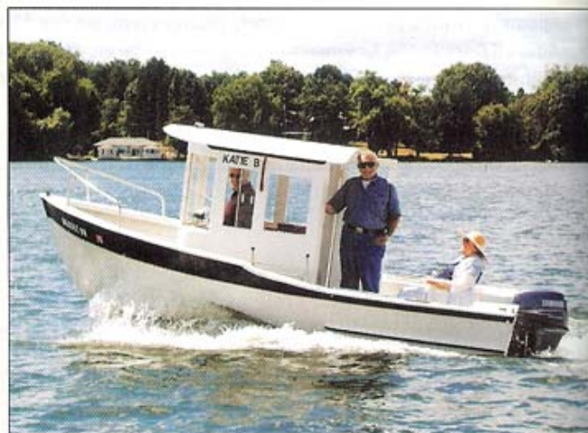
Above —KATIE B is Dick Rosen's interpretation of the Sherwood Queen design from Glen-L Marine. She's a miniature tug, 15'6" overall with a 7'4" beam. Dick modified the cabin, using automotive glass and installing a door. KATIE B is made of marine-grade plywood and lots of sealer and marine paint; no fiberglass or epoxy was used in construction. The owner tells us she is "dry as a bone." Powered by a Yamaha four-stroke, high-thrust, 25-hp motor, she will be used for fun and adventure in the lakes of Ohio, particularly Sandusky Bay and Lake Erie. Plans are available from Glen-L Marine, 9152 Rosecrans Ave., Bellflower, CA 90706; 562-630-6258; < www.Glen-L.com >.
