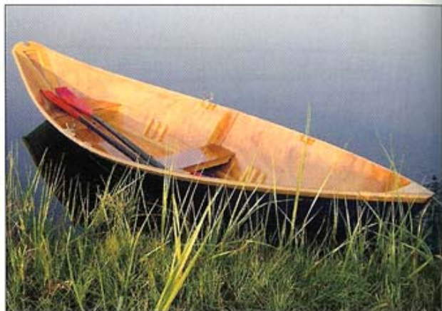
Above —Guided by the book How to Build the Gloucester Light Dory , by Harold "Dynamite" Payson, first-time boatbuilder Matt Camisa built this Phil Bolger-designed Gloucester Light Dory of okoume plywood over white-oak framing. Matt sheathed the bottom in 6-oz fiberglass cloth coated with epoxy and finished the boat with varnish and paint. The builder reports: "She looks great and rows even better. It turns heads every time I take it out." Plans for the Gloucester Light Dory and accompanying book are available from < www.instantboats.com >. The book is also available from The WoodenBoat Store.
