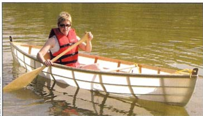
Above —CANARY, named for the first airplane owned by the builder's hero, Amelia Earhart, is a 10'6" skin-on-frame ultralight solo canoe. The builder, Carin Mincemoyer, used ash for stringers and gunwales, white oak for the ribs, plus nylon lashing and ballistic nylon skin, coated with polyurethane. She also carved the paddle, made of yellow poplar. Carin intends to paddle the canoe exploring rivers and lakes near her home in Pittsburgh. You can contact the designer, Brian Chandler, at 1362 E. 33rd Ave., Vancouver, BC, V5V 3B7, Canada; < www.dreamcatcherboats.com >.
